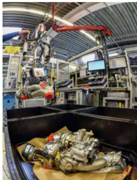
Using a crane, the worker positions the turbochargers in the trays of the four boxes after the final assembly station.
