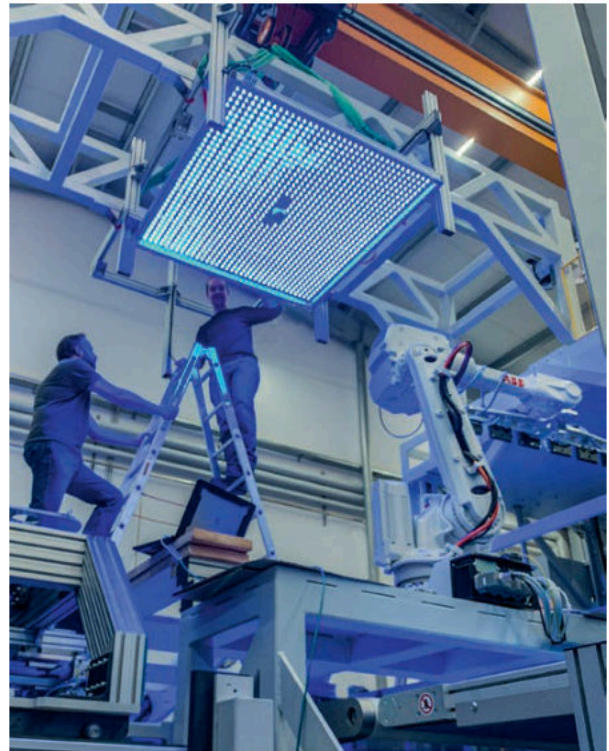
The homogeneous light of a 1,500 × 1,500 mm LED light enables precise surface inspection with reliable detection at a resolution of 0.3 mm.
