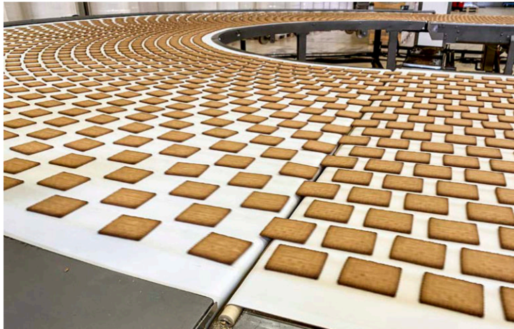
Figure 2 | 4,200 biscuits per minute must be inspected very precisely for many quality features and classified as pass or fail.
