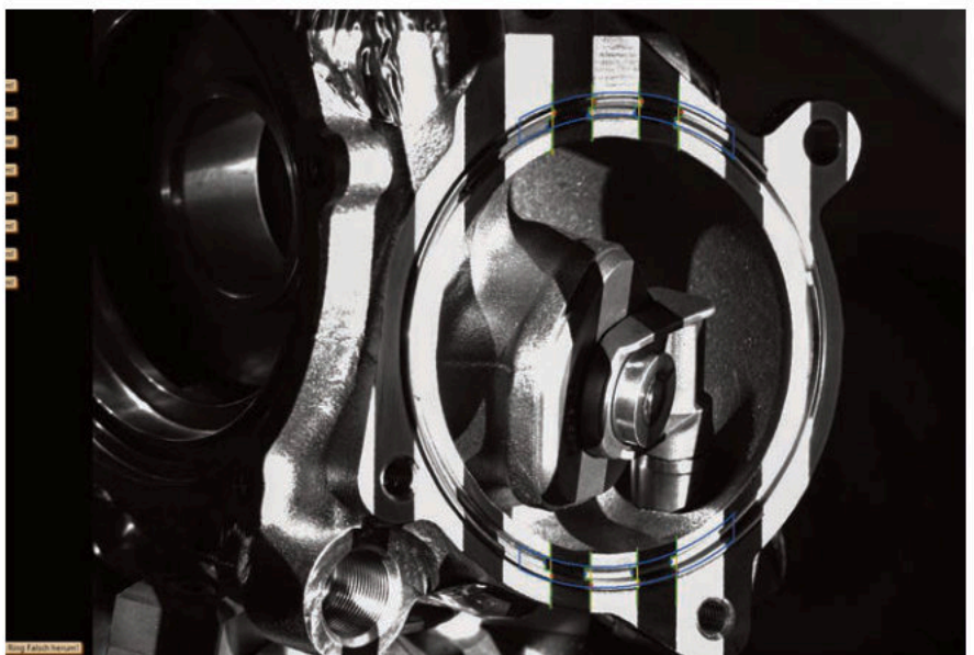
The Z-ring of the turbocharger assembly is checked for presence and 3D height using an LED projector and a 20 MP zoom camera.
