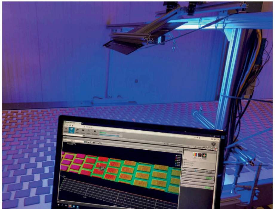
Designing the complex vision system for biscuit production involves capturing many relevant inspection functions. Image: Cretec.
