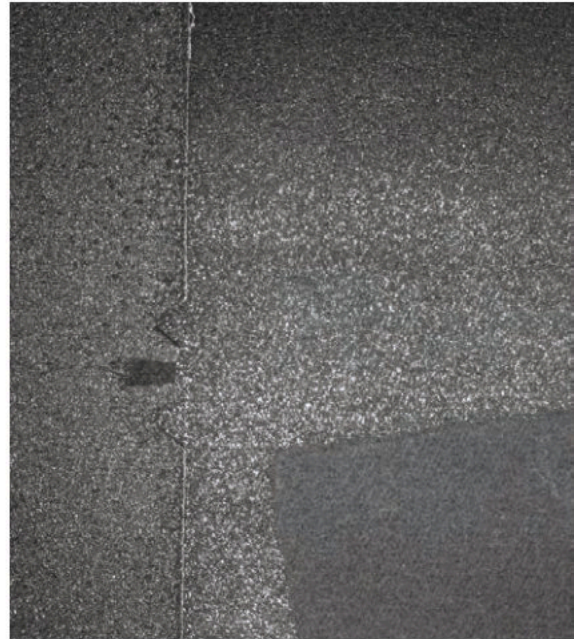
The camera of the vision system captures defective adhesive application in great detail.
