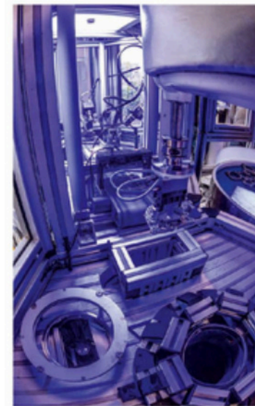
2 | The robot grips the parts precisely and presents them to the 2D and 3D vision systems for checking dimensions and surface condition. © Cretec
