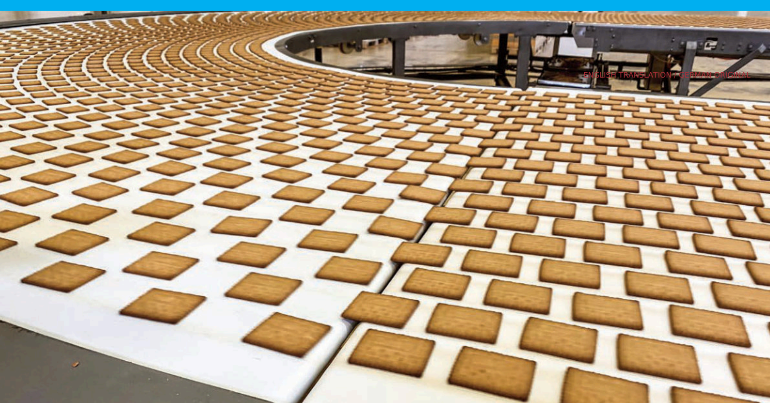
Figure 1 | During production, 4,200 biscuits per minute must be inspected precisely for over 20 features and sorted into pass/fail categories. Many results are used directly as a data stream, feeding back into ongoing production.
