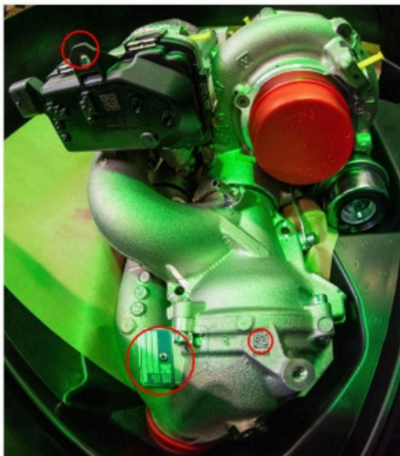
Three of the twelve features stand out: a 3 mm-wide plastic web, the nameplate and the approximately 5 mm × 5 mm DataMatrix code.
