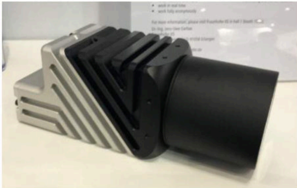
Fig. 3: Baumer's AX camera, based on an open-source Linux platform, integrates a high-performance NVIDIA GPU (Jetson TK1/TX2).
