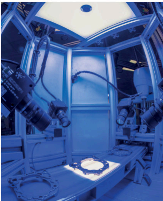
03 | Five high-resolution cameras inspect many features simultaneously in a very short time using reflected and transmitted light on the moving conveyor.
