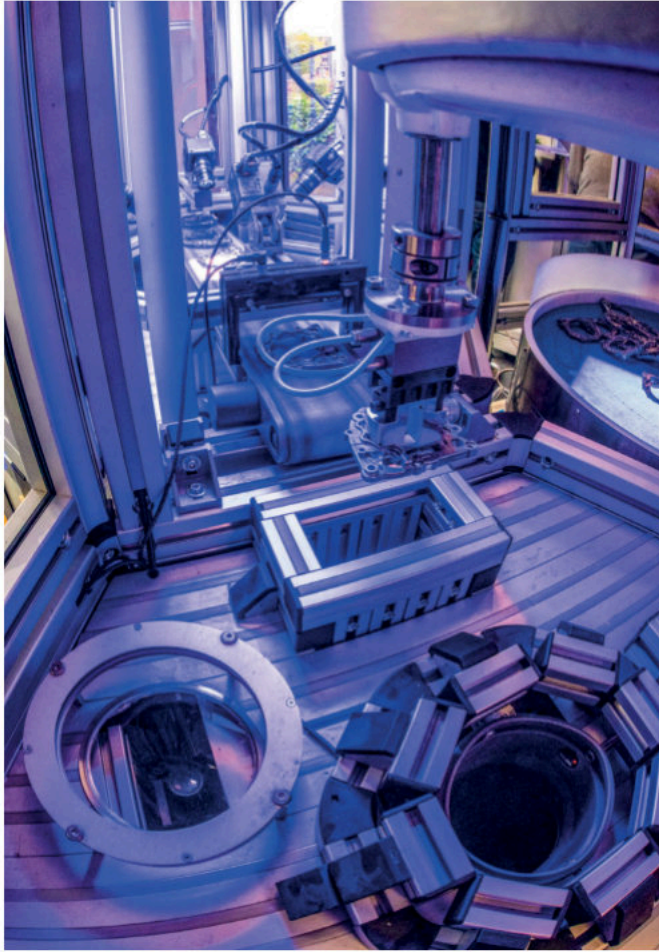
01 | A complex, flexible inspection system with a minimal footprint. Each part is inspected automatically and precisely from all sides (360°) for 21 features. Data and images are documented and the parts are sorted into pass/fail categories.
