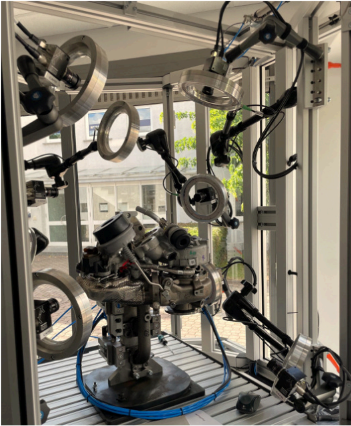
The eight 5 MP cameras and their individual high-resolution fields of view provide complete all-round 3D inspection of the turbocharger assemblies. (Image: Cretec)
