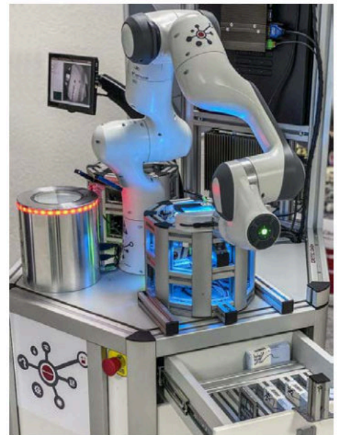
The modular QBIC system is a universal, highly flexible work platform that can perform many different inspection tasks fully automatically in minimal space. (Photo: Cretec)
