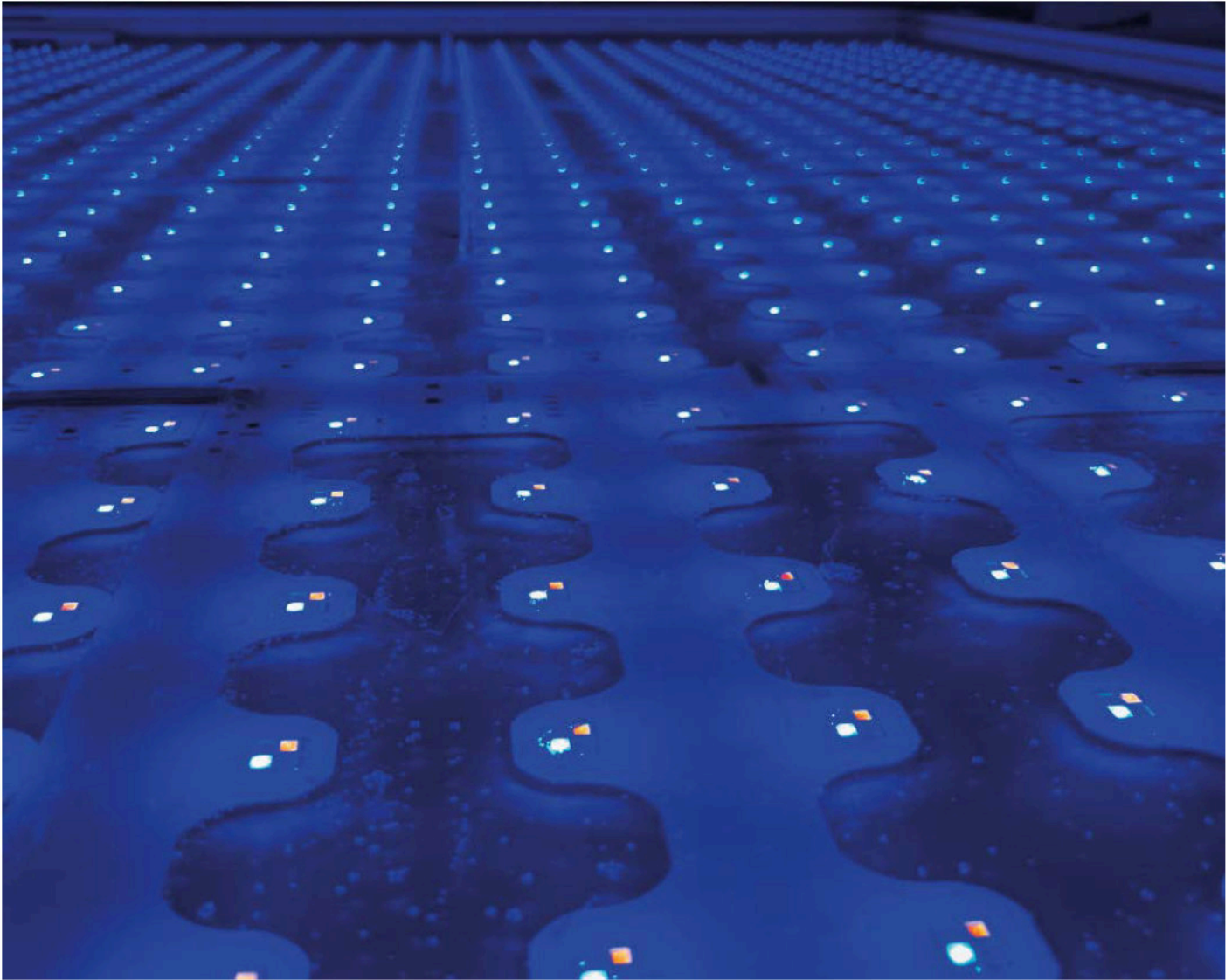
Large-area lighting modules with four-colour LEDs in strobe, colour-change or daylight mode enable a wide range of industrial machine-vision applications.
