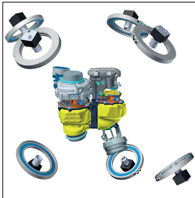
03 The eight 5 MP cameras are positioned so that their individual high-resolution fields of view provide complete all-round 3D inspection of the turbocharger assemblies.
