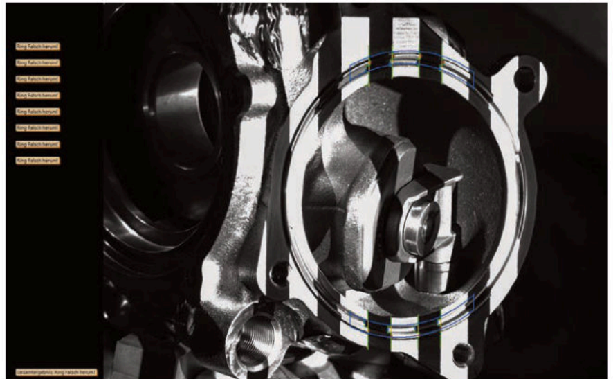
Figure 2 | The Z-ring of the turbocharger assembly is checked for presence and 3D height using an LED projector and a 20 MP zoom camera.
