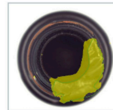
Figure | HALCON anomaly-detection technology with self-learning detects defects in the bottle neck. © Cretec / MVTec
