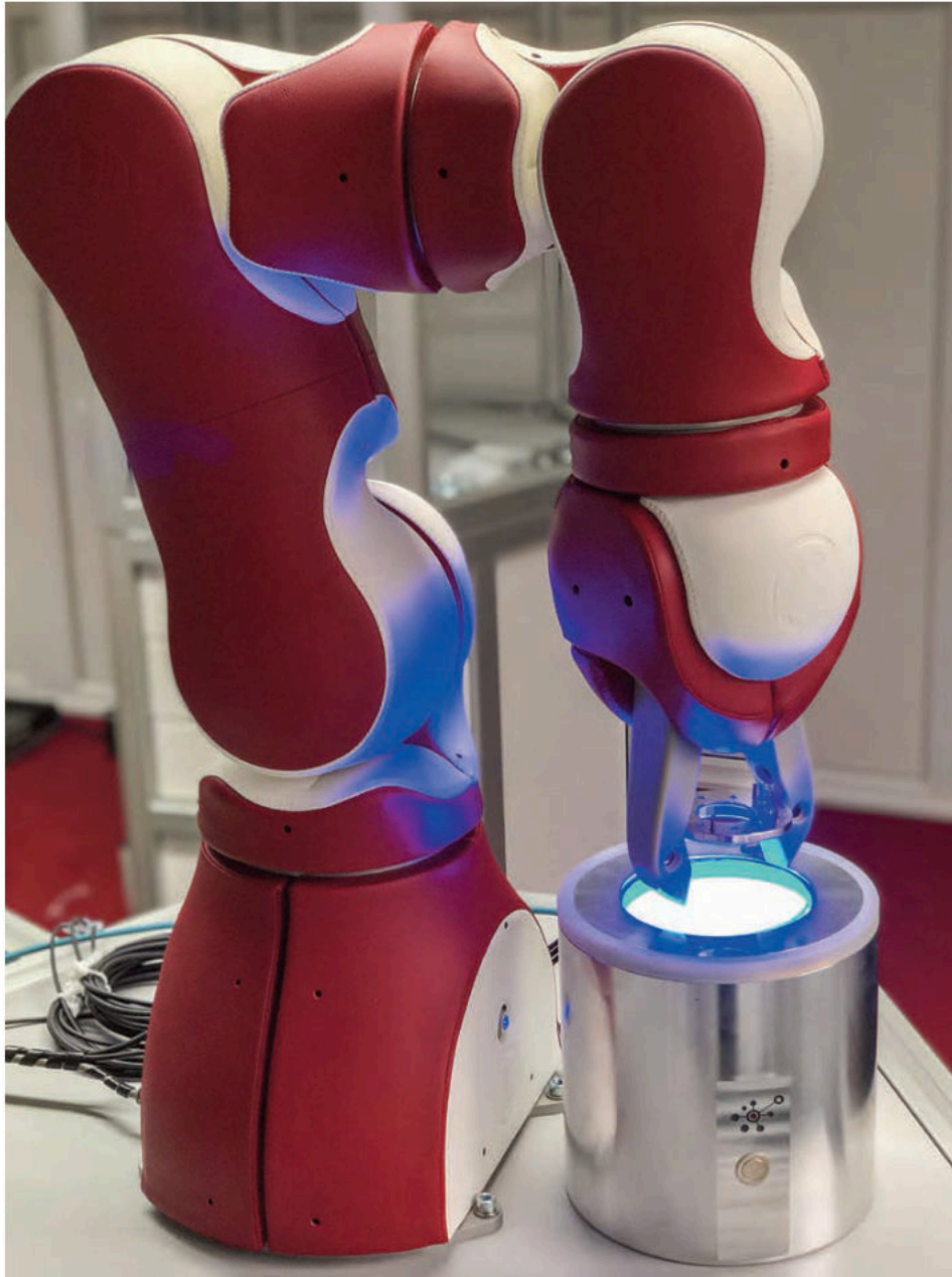
Fig. 4: VisionTube can also be used in fully automatically controlled manufacturing cells or combined with a collaborative robot.
