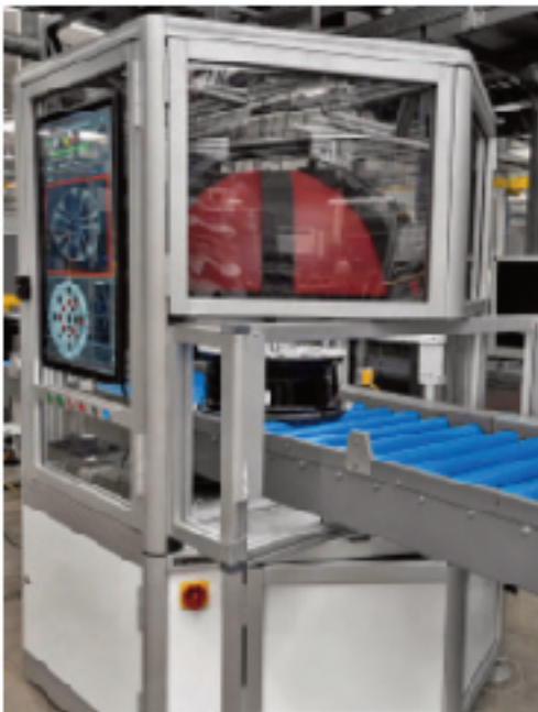
Integrated with the conveyor, QBIC Wheels performs final quality inspection of wheels in a cycle time of less than 6.2 s.
